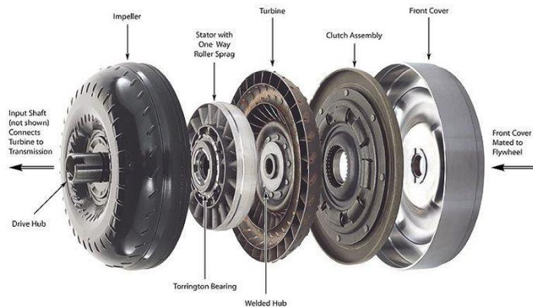
Gambar 3. 34 *Torque converter*
