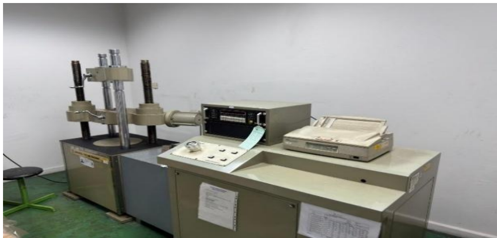
Gambar II. 2 Universal Testing Machine GT-7001-L10/EMERL0034 (Sumber : Dokumentasi Pribadi)
